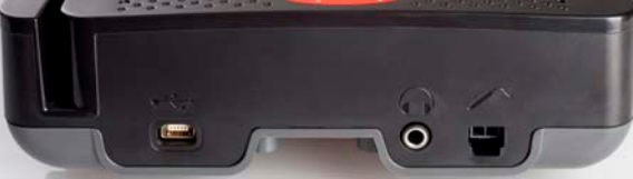
Figure 2: iSC250 Peripheral Ports
