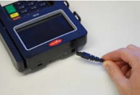
Figure 1: Inserting the stylus connector into the stylus port
