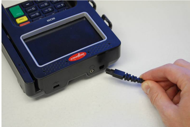
Figure 5: Inserting the stylus connector into the stylus port
