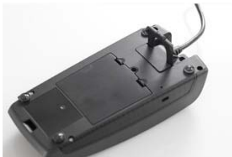
Figure 4: Cable placed in iPP300 port
