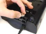
Figure 1: Unscrewing the Thumbscrew
