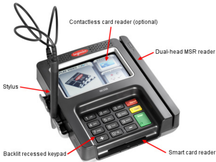
Figure 1: iSC250 Device Parts (front)
