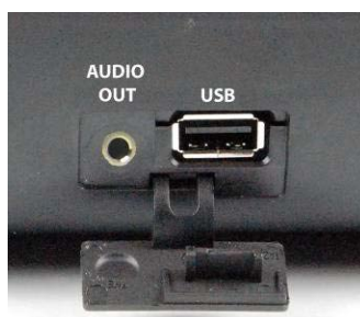
Figure 10: iSC350 Side Ports
