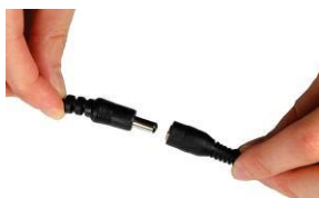
Figure 11: Connecting a Power Supply
