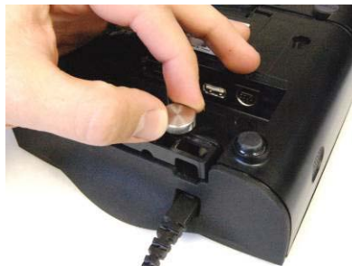
Figure 5: Unscrewing the Thumbscrew
