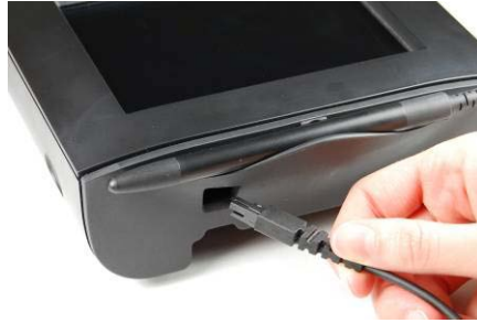
Figure 6: Inserting the stylus connector into the stylus port
