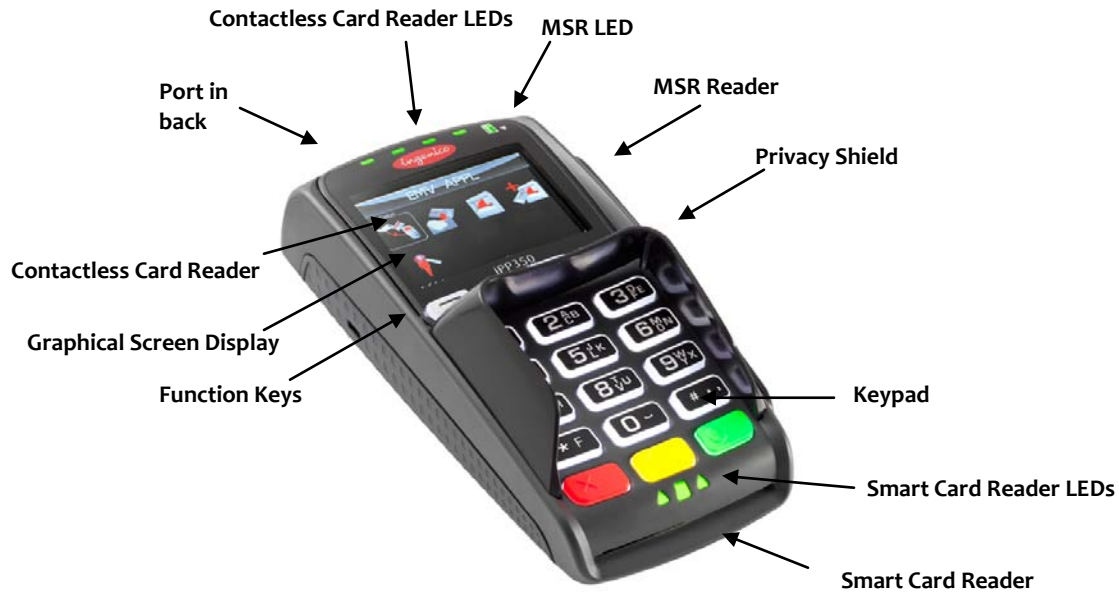
Figure 1: iPP300 Device Parts
