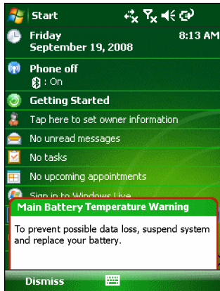
Figure 2-9 Main Battery Temperature Warning Dialog Box
